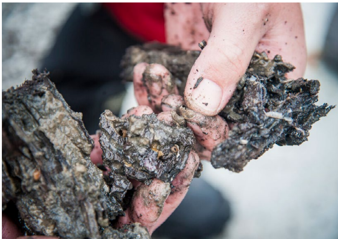
04. Wooden shipwrecks that are exposed at the bottom surface are eaten by naval shipworms (Photo: Martijn Manders)
